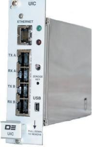
The UIC board incorporates one RJ-45 connector for the (Ethernet 10/100 Base-T) connection to the outside world and four RJ-45 connectors, for supporting two Receivers and two Transmitters stationed in the subrack. The USB connection is for connection to a maintenance / programming PC, allowing firmware updates via flashing. (In the future, updates will be downloadable from the Daniels Electronics website.)
